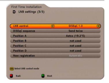
Press the ▲▼ buttons to switch to "DiSEqC sequence". Select how often the DiSEqC™ command is to be sent using the ◀▶ buttons.
